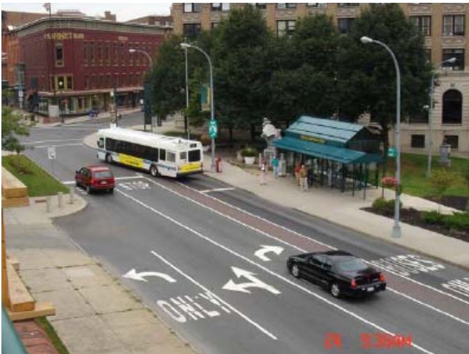
Bus moving into the intersection after receiving the "queue jumper" indication
